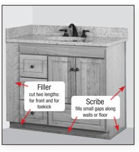
Cut Filler or Scribe to length and secure in place with adhesive or fasteners of your choice.
